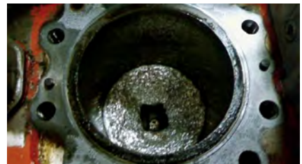
Damage to valve, cylinder, and piston occurred prior to VSM installation.
